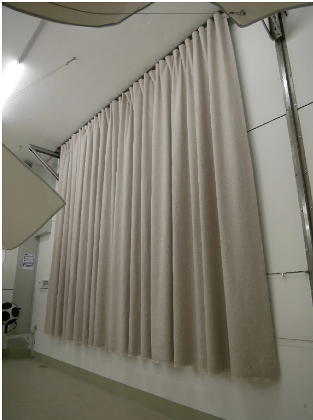
Figure B.2. Test object mounted in the reverberation room, diagonal view.
